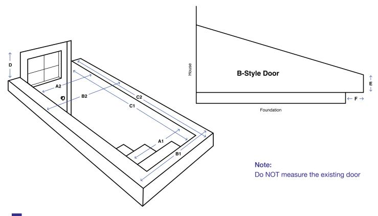
Use the following illustration as a guide to assist you while you take the required measurements listed below. The B-Style door comes with a raised threshold to accommodate higher grade.
